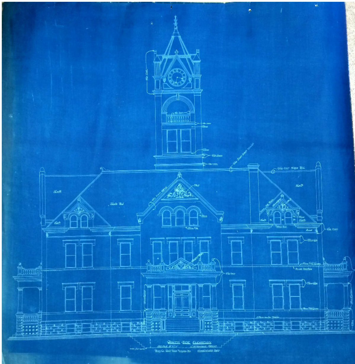
Figure 6. 1904 Perry County Courthouse Plans by J.W. Gaddis, South Elevation. Source: Perry County Courthouse archives.
